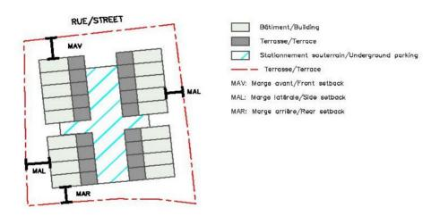
iii)Plan C: Siting of eight (8) buildings on a single lot with an underground parking garage and an outdoor terrace:
